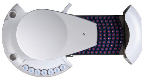
The EL3200A features the innovative SyringeID, a proprietary technology<sup>1</sup> based on RFID tags. The SyringeID is able to identify syringes in an univocal way; thereby preventing errors when mounting a syringe, preventing syringe volume mismatching and keeps track of the syringe consumption (preventive maintenance counters). The SyringeID system is able to provide you with a level of confidence never previously achieved by identification systems based on syringe carriers.
